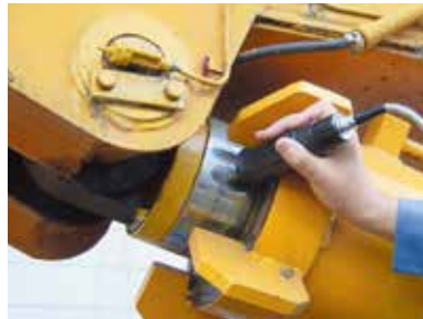
● Diagnosing wear and tear using hardness measurements
